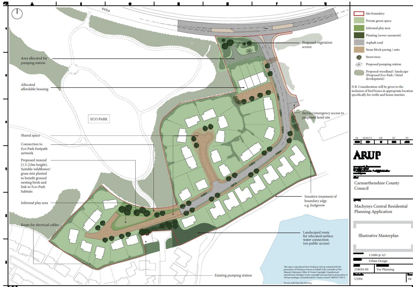
Figure 5: Detailed map of the Illustrative Masterplan of the proposed Residential development, showing the locations of buildings, play area and possible pumping station. Provided by ARUP
