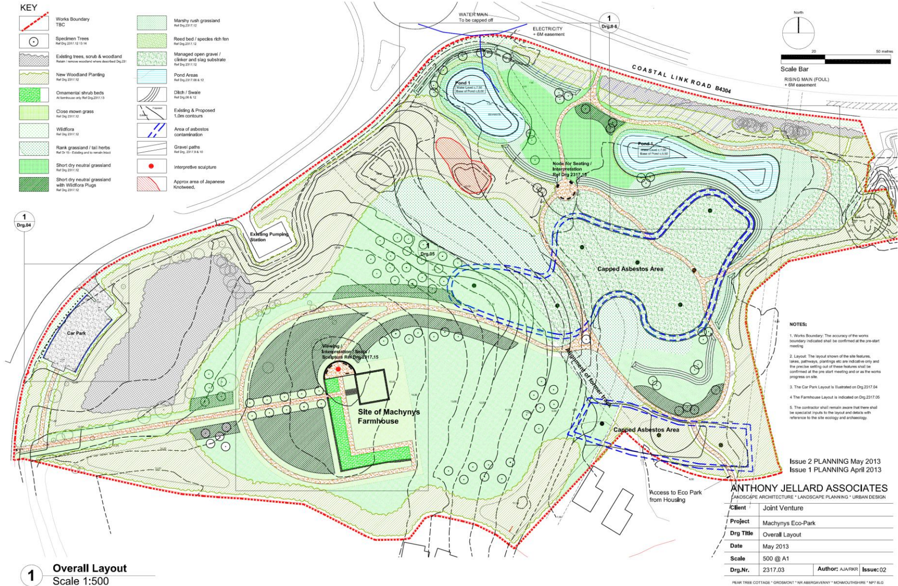
Figure 4: Detailed map of the layout of the proposed Eco-Park, showing proposed landscape profile, planting, pathways, car park and site of Machynys House provided by ARUP on behalf of the client
