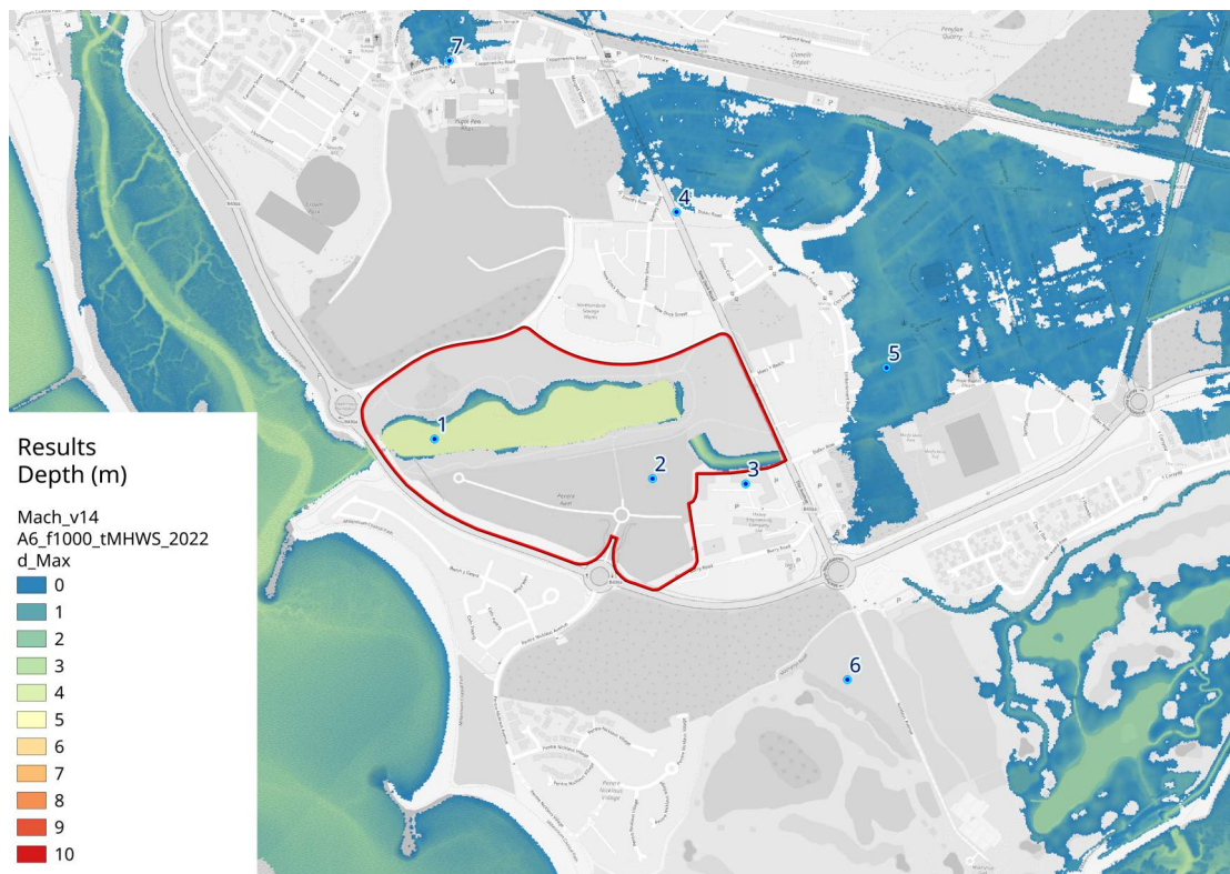
Figure 4.15: Pre-development Results Peak Water Depth for a 0.1% AEP fluvial event in conjunction with a MHWS tidal surge in 2022
