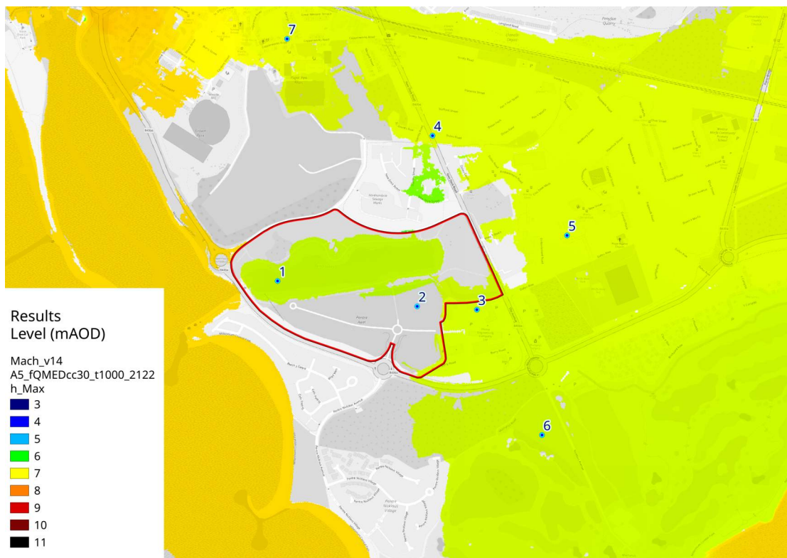
Figure 4.3: Pre-development Results - Peak Water Level for a 0.1% AEP Central tide surge event in conjunction with a QMED fluvial flow with a 30% allowance for fluvial flow in 2122
