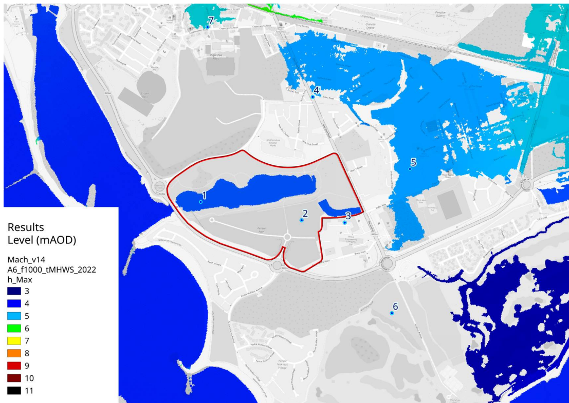
Figure 4.7: Pre-development Results Peak Flood Level for a 0.1% AEP fluvial event in conjunction with a MHWS tidal surge in 2022
