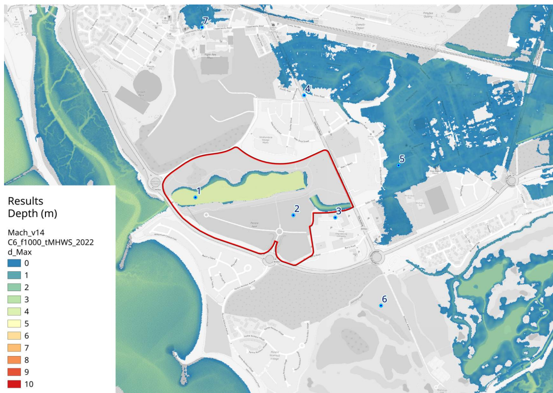
Figure 4.17: Post-development Results Peak Water Depth for a 0.1% AEP fluvial event in conjunction with a MHWS tidal surge in 2022
